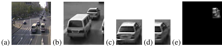
Fig. 4. The tracking result during occlusion. (a) The frame containing the occlusion. (b) The rectangular area containing the object to be tracked. (c) The object block. (d) The right sub-part. (e) The tracking result of the right sub-part.
