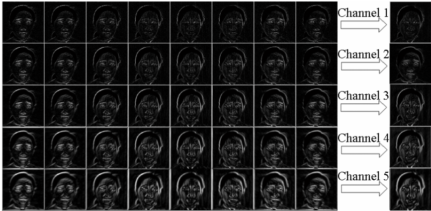
Fig. 2. Responses of the Gabor filters and the representative images for all 5 scales(right)
